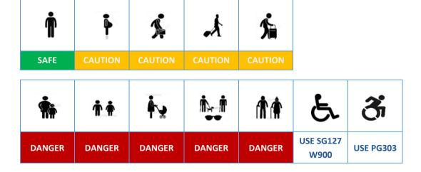
If regular use by user types with the risk classification of caution or danger is anticipated, than we recommend that the optional detection sensors are fitted, all parameters are set to the optimum level of protection and additional safety signage may be required.
