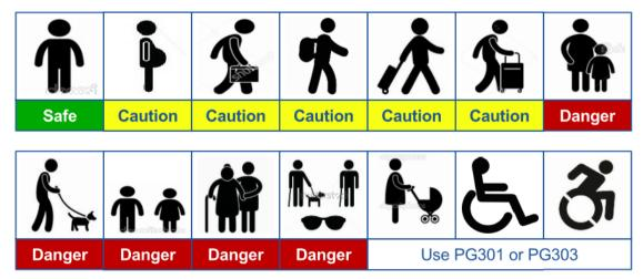
If regular use by user types with the risk clarification of caution or danger is anticipated, than we recommend that optional extra photocells are fitted and all parameters are set to the optimum level of protection.
