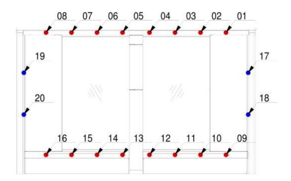
Cells 01 to 16 are supplied as standard, all cells are transmit and receive. The signal emitted by the transmitter cell (left gate, in direction A) is received by the receiver cell on the right gate. The cell beams are laid out in a horizontal group.
