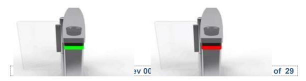
The functional LEDs are a green arrow and red cross fitted on the top cover at either end of the lane. When a valid open command is received the green arrow will light showing it is safe to pass, and the opposite end of the lane the red cross will illuminate showing it is not safe to pass.
